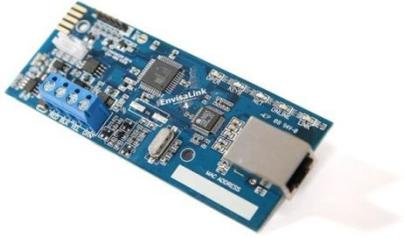
This application note outlines how to use the **Envisalink**'s built-in Syslog client to log security events to a LAN connected Syslog server. It also explains how to install an open-source Syslog server on a Windows PC for those who don't have a Linux Syslog server. The Syslog client is only available on the **Envisalink 4** and requires a firmware version of 1.01.108 or higher.
